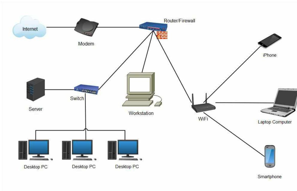
Note: the modem & Internet aren't part of the LAN - they are just showing how a LAN could be connected to the Internet (though LANs can also be air-gapped (not connected) to the Internet too)
